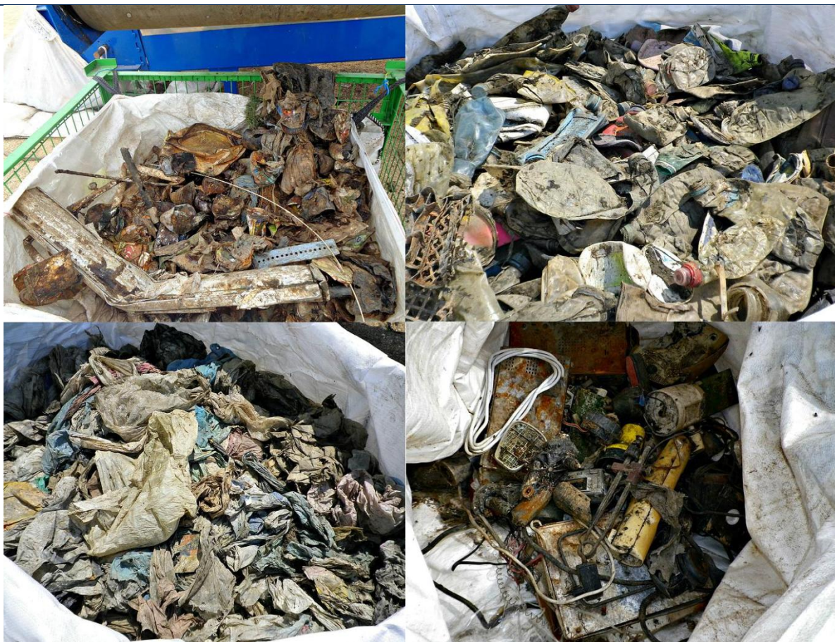
Figure 4.3.1-5: Pictures of separated waste streams from the PL contents: ferrous metallic waste, hard plastics, film and membranes and a few E-waste (LIFE reclaim project)
