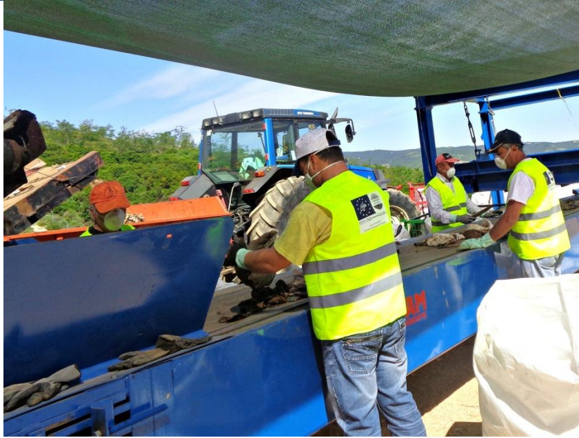
Figure 4.3-5: Hand-sorting workers: a difficult but most necessary job during LFM (LIFE reclaim project).
