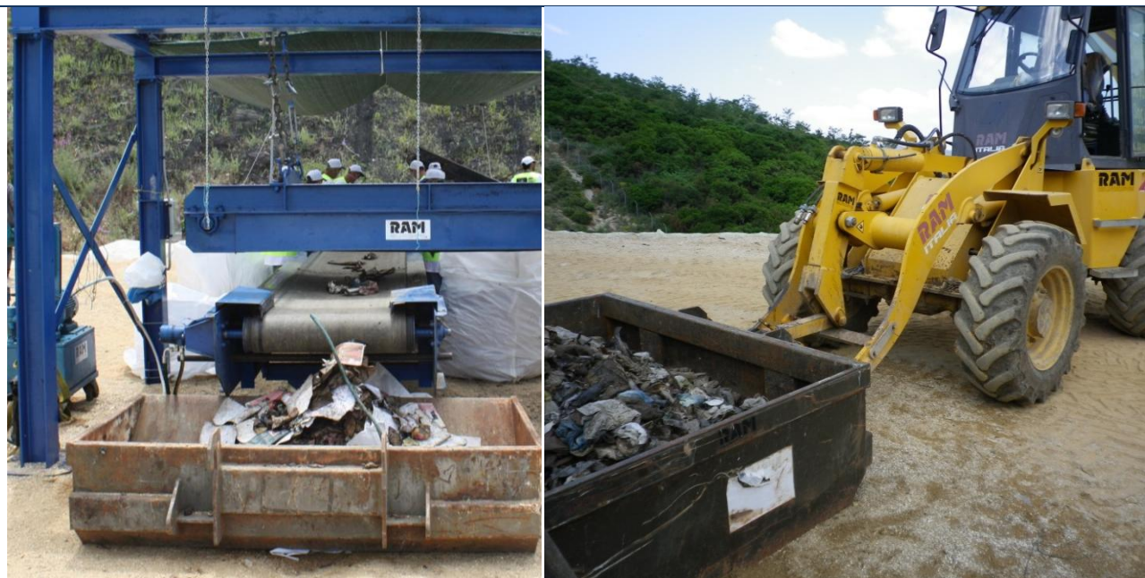
Figure 4.3-3 and 4: Updated collection of the residual material at the end of the membrane, using a special skip (LIFE reclaim project)
