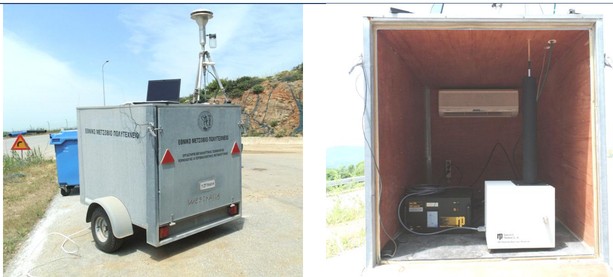
Figure 6.3. Set-up location of the TEOM PM-10 monitoring unit.
