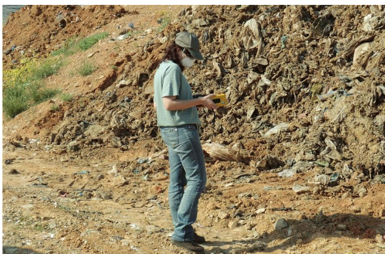
Figure 6.4. Monitoring gaseous emissions at the waste excavation area.
