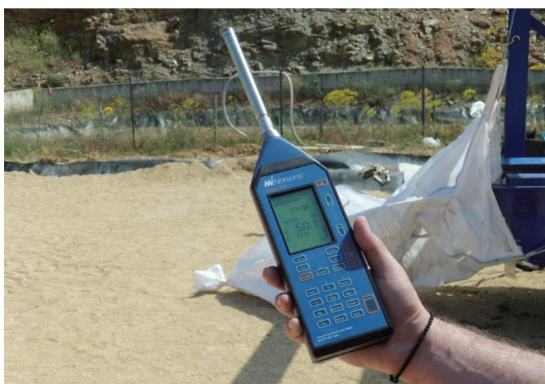
Figure 6.5. Monitoring sound pressure level (SPL) at the waste processing area.
