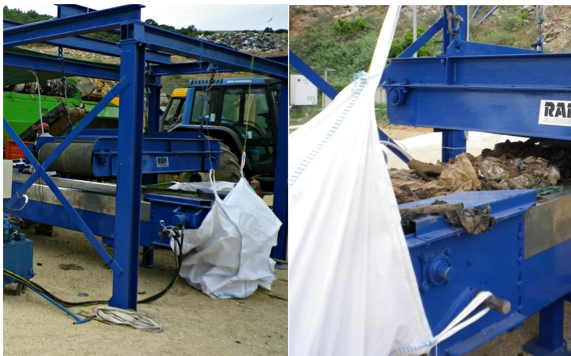
Figure 4.3-1 and 2: Collection of the residual material at the end of the membrane, using a BB (LIFE reclaim project)
