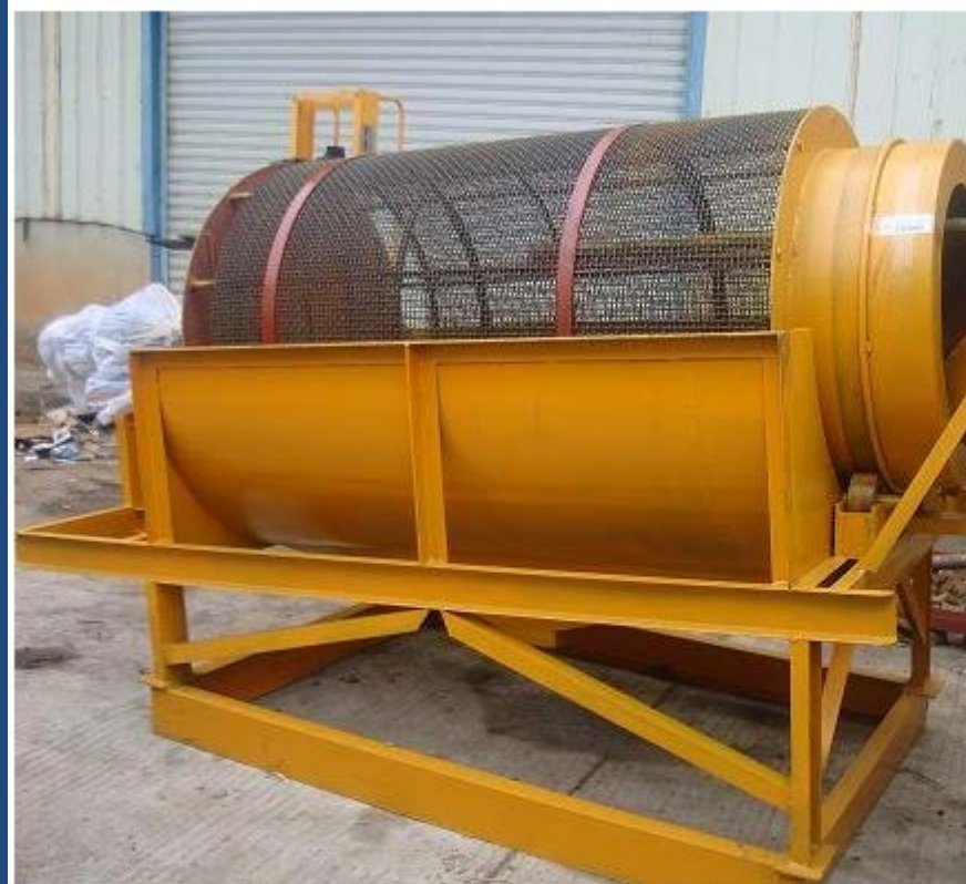
Figure 8. Revolving screen used in trommels:
